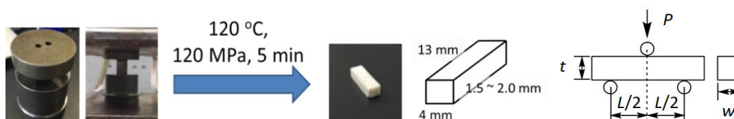
Fig. 4. Mold of composite powder by hot press and three-point-bending test
