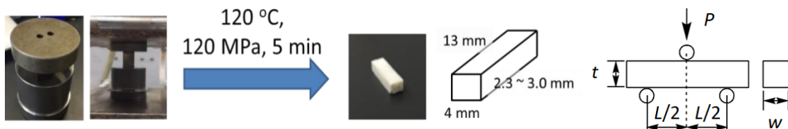
Fig. 3. Mold of composite powder by hot press and three-point bending test.
