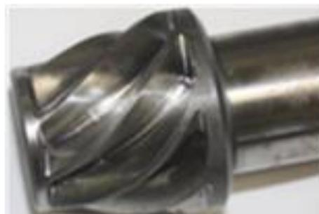
Fig. 2-2 Proposed pinion fabricated by five-axis controlled machining center
