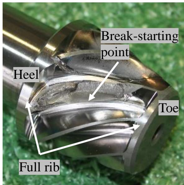
Fig. 4-1 A proposed spiral bevel gear after a fatigue test with full rib
