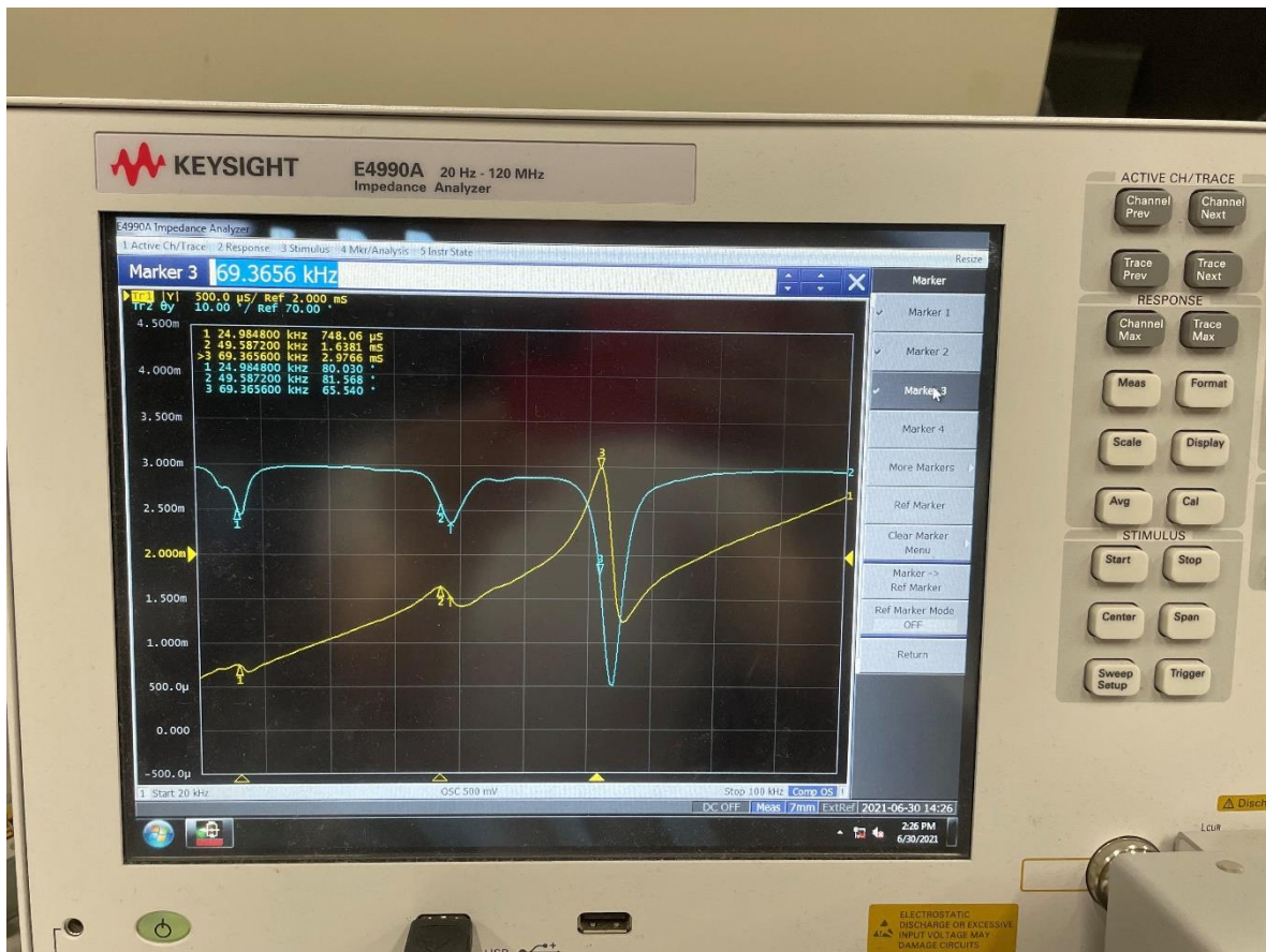
Figure 4.6 Impedance Analyzer (E4990A) during measurement of the resonance frequencies of an ultrasound liquid crystal lens
