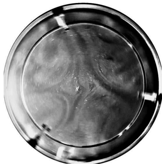
Fig. 7. A photograph illustrating the flow pattern on top plane with an azimuthal wave number of 4 (at Ro_T = 5.1\times 10^{-3} and Ta = 1.44\times 10^9 ).
