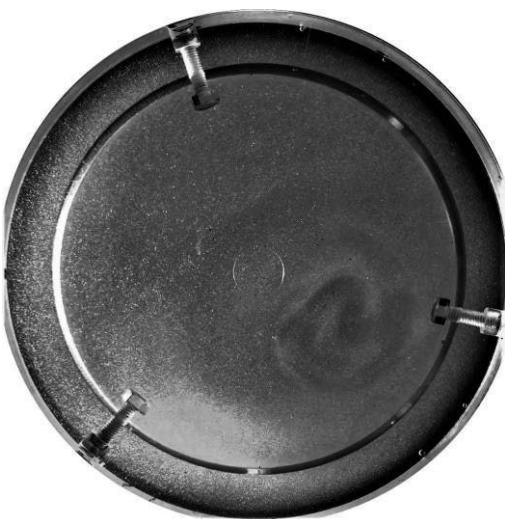
Fig. 5. A photograph illustrating the flow pattern on top plane with an azimuthal wave number of 1 (at Ro_T = 6.8 and Ta = 2.83\times 10^7 ). An eccentric vortex corresponds to the wave number of 1.
