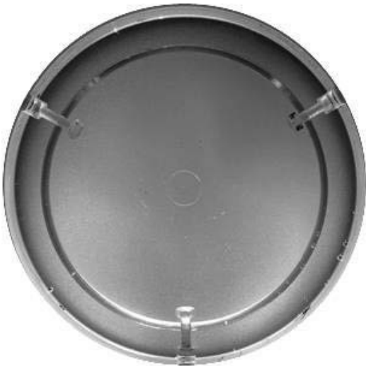
Fig. 4. A photograph illustrating the flow pattern on top plane with an azimuthal wave number of 0, in lower symmetrical régime (at Ro_T = 1.26 and Ta = 3.25\times 10^6 ).
