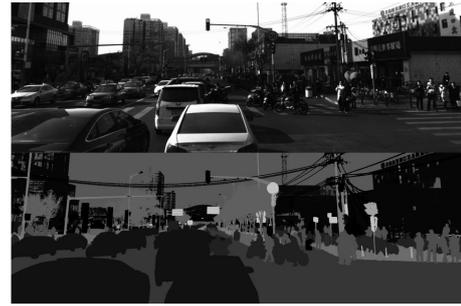
Fig. 1. Semantic segmentation for self-driving.<sup>7)</sup>
