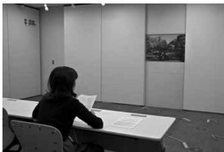
Fig. 3. Experimental environment constructed with 12 ceiling lights and the Virtual Window.
