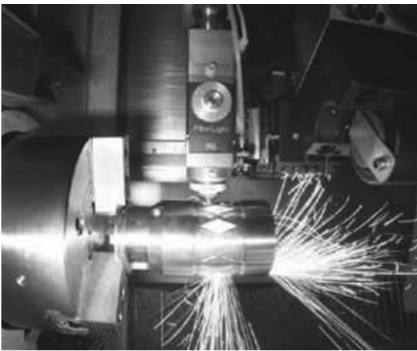
Fig. 8. Cutting performance with a fiber laser.
