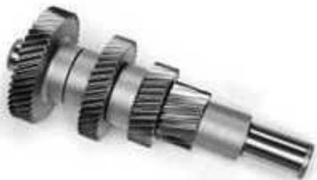
Fig. 4. Machined gear blank with a turning center.
