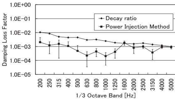
Fig. 12. Damping loss factor comparison result of decay ratio method and power injection method
