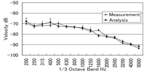
Fig. 4. Estimation result of vibration response
