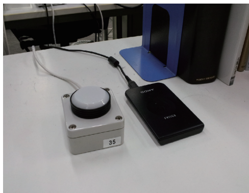
Fig. 7. Illuminance sensor and IC card reader.
