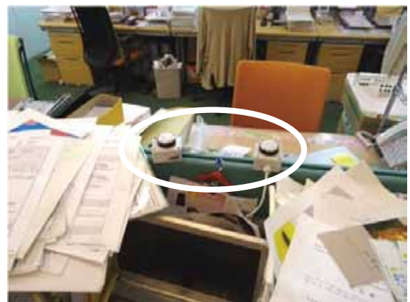
Fig. 3. A situation prohibiting the placement of an illuminance sensor on the workplane (example).
