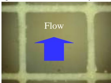
Figure 3. A cell in the innards of a catalytic converter.
