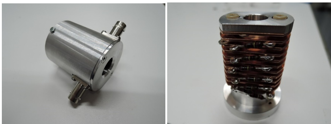
FIGURE 4.1: (Left) Image of the actual mobility spectrometer, and (Right) the spectrometer device without the outer ground chassis.
