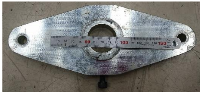
(b) The element of clamping sample of the impact device.
