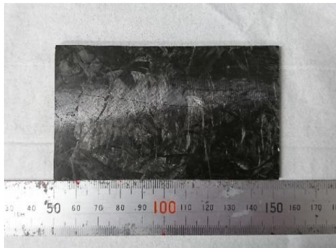
The Fig. 4-2. The representative image of sample for impact test.
