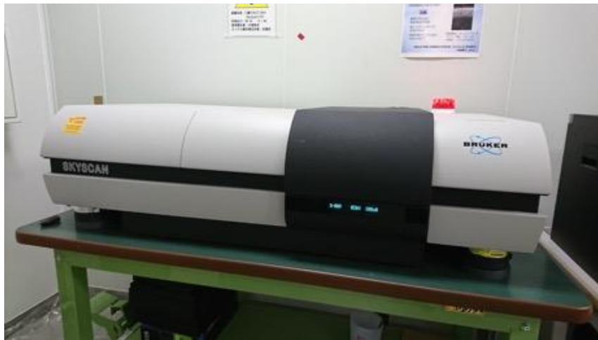
The X ray CT scan (Skyscan MicroCT - Brucker)
