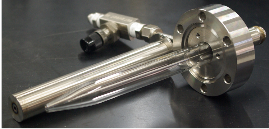
Fig. 2.7. A photograph of the 1st gen CCP type atomic source apparatus.
