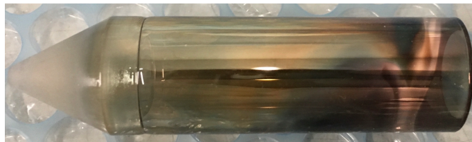
Fig. 3.4. A photograph of the quartz tube which has a 1 mm diameter orifice after the first operation.
