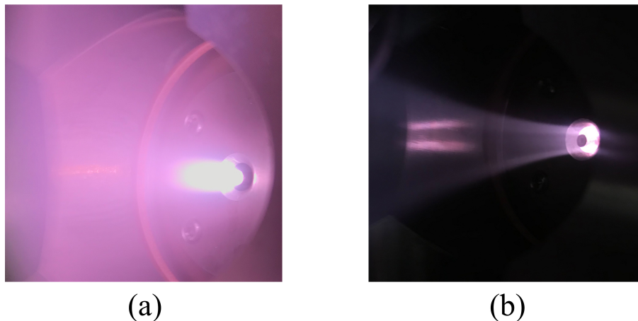
Fig. 3.11. Photographs of the plasma produced in the 4th gen CCP source. (a) Plume mode (b) Out of the plume mode.
