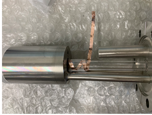
Fig. 2.21. A photograph of the spiral antenna insulated by a quartz tube after the transmission coaxial line removal.
