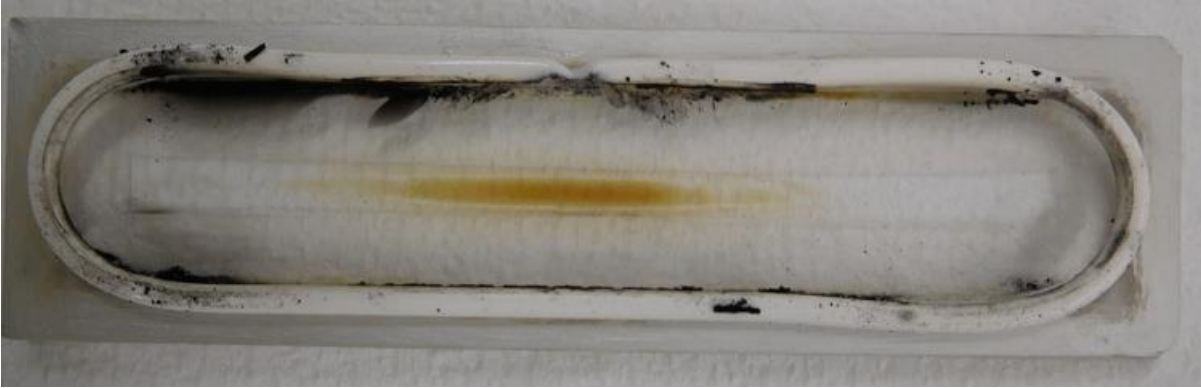
Figure 4.1: Image of the burnt quartz window and rubber O-ring seal.
