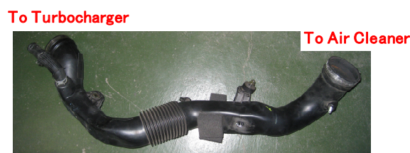
Fig.4-5 Conventional Intake Pipe
