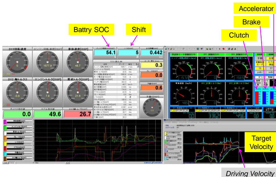
Fig.7-10 Picture on the screen of Hybrid Powertrain Test Bed System
