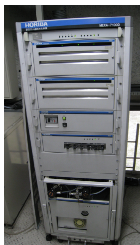
(a) Exhaust-gas Measurement System
