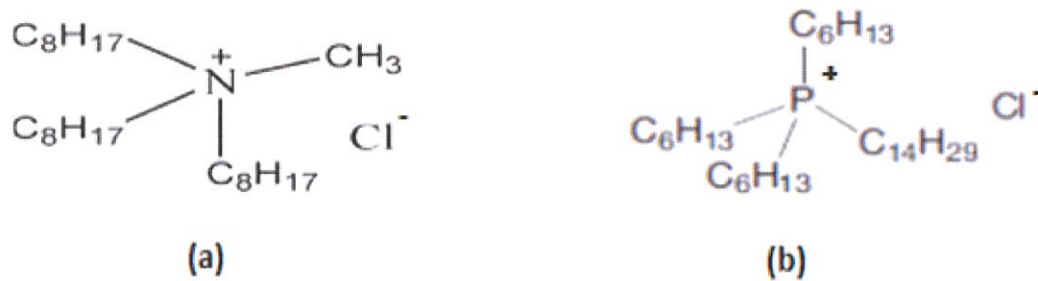
Figure 1. Molecule structures of ILs used: (a) Aliquat 336 ( N -Methyl- N,N,N -trioctylammonium chloride) and (b) Cyphos IL-101 (Trihexyl(tetradecyl)phosphonium chloride)
