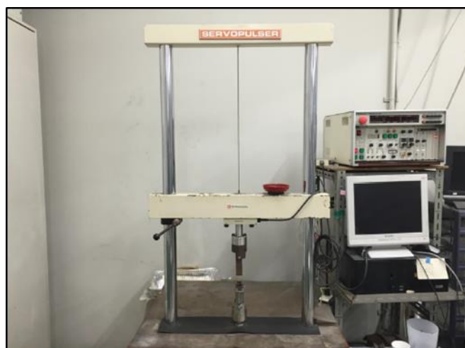
Fig. 4-10 Apparatus for three-points bending fatigue tests.
