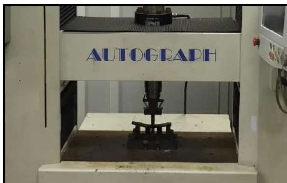
Fig. 3-9 Apparatus for three-point bending tests and fracture toughness tests.
