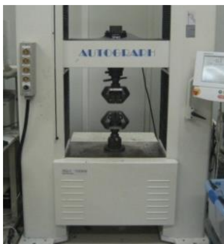
Fig. 3-8 Apparatus for static tensile tests.
