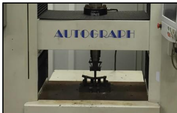
Fig. 4-8 Apparatus for static three-points bending and ENF tests.
