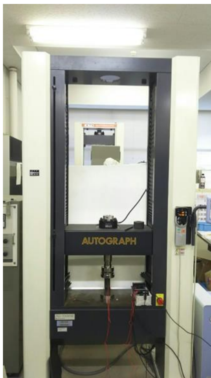
Fig. 4-5 Apparatus for compression tests.
