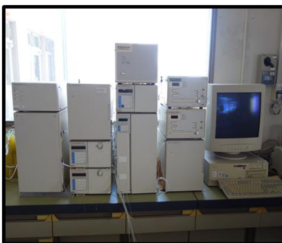
Fig. 2-12 Apparatus for measurement of weight-average molecular weight of matrix. (Gel Permeation Chromatography; GPC)
