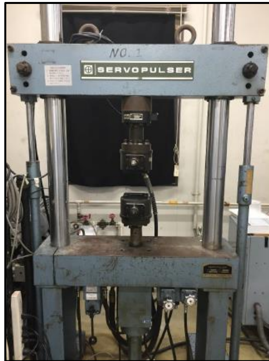
Fig. 3-15 Apparatus for tensile fatigue test.
