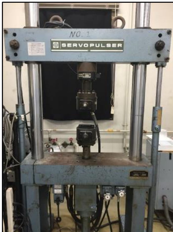
Fig. 2-16 Apparatus for measurement of \tan\delta test.
