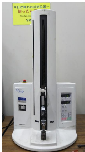
Fig. 2-17 Apparatus for static tensile test of model specimen.
