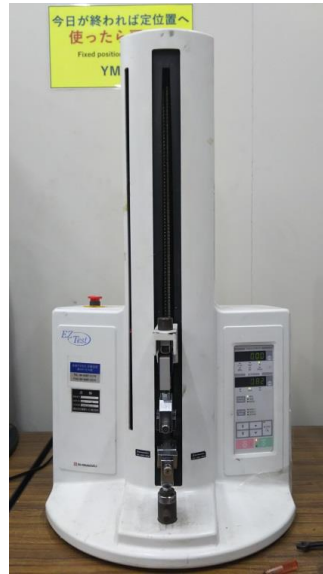
Fig. 3-13 Apparatus for static tensile test of model specimen.
