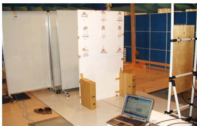
Fig. 6.14 Photograph of experimental set up for measurements of tag reading rate shown in Fig. 6.13.
