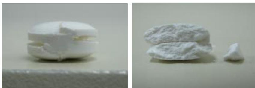
Figure 6-3 Failure patterns of tablets with a capping tendency after the diametrical compression test.
