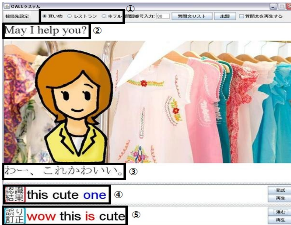
Figure 4.2: A screenshot of the CALL interface: (1) dialogue scenario selection (shopping, restaurant and hotel); (2) prompt by system; (3) hint stimulus; (4) recognition result; (5) corrected feedback
