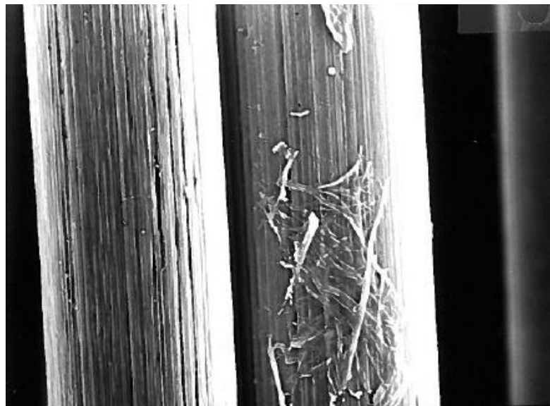
Figure 3.12 : SEM photograph after excessive treatment in NaOH aqueous solution
