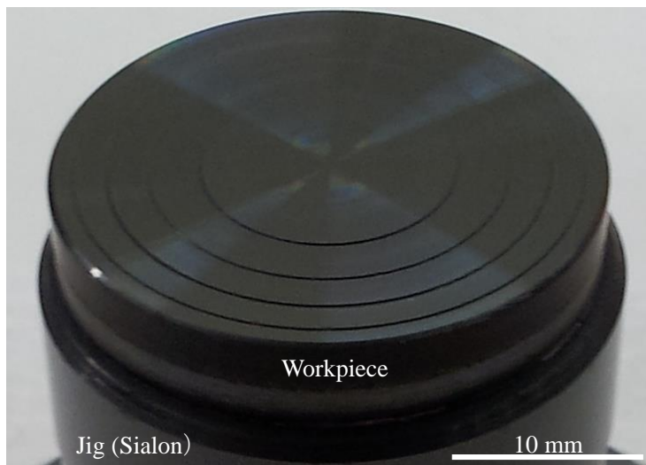
Fig. 3.13 Photograph of machined Fresnel mold.
