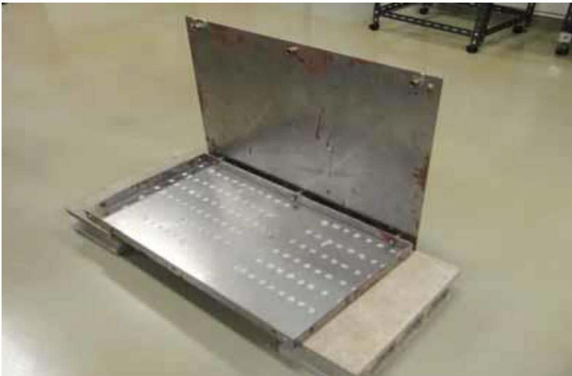
Figure 5.13 View of L-shaped partial structure of enclosure
