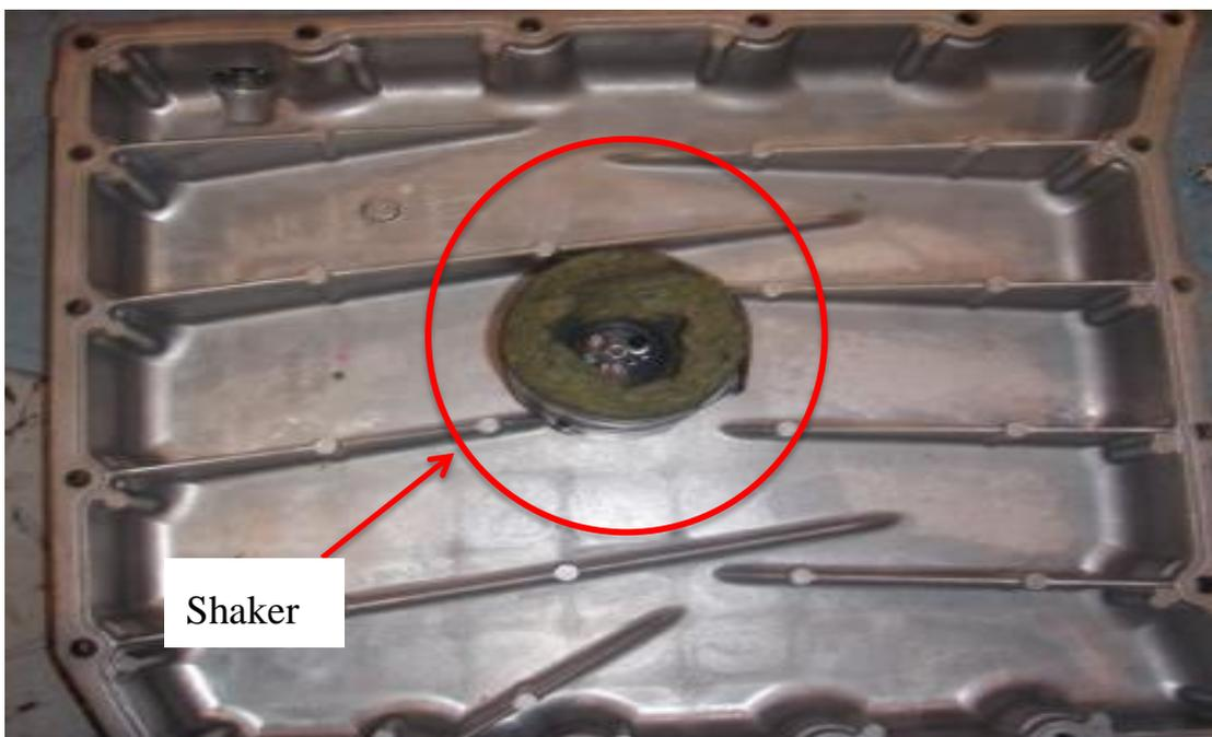
Figure 2.1 Oil pan inside view for speaker test (upper) and shaking test (lower)
