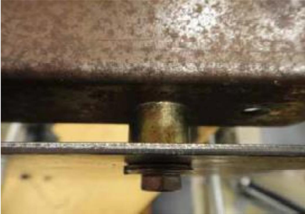
Figure 5.14 Detailed view of bolt and spacer connection
