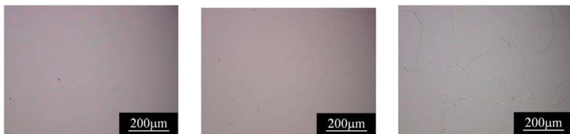
(a) 120 s, thickness=0.4 μm (b) 240 s, thickness=1.0 μm (c) 360 s, thickness=1.1 μm
