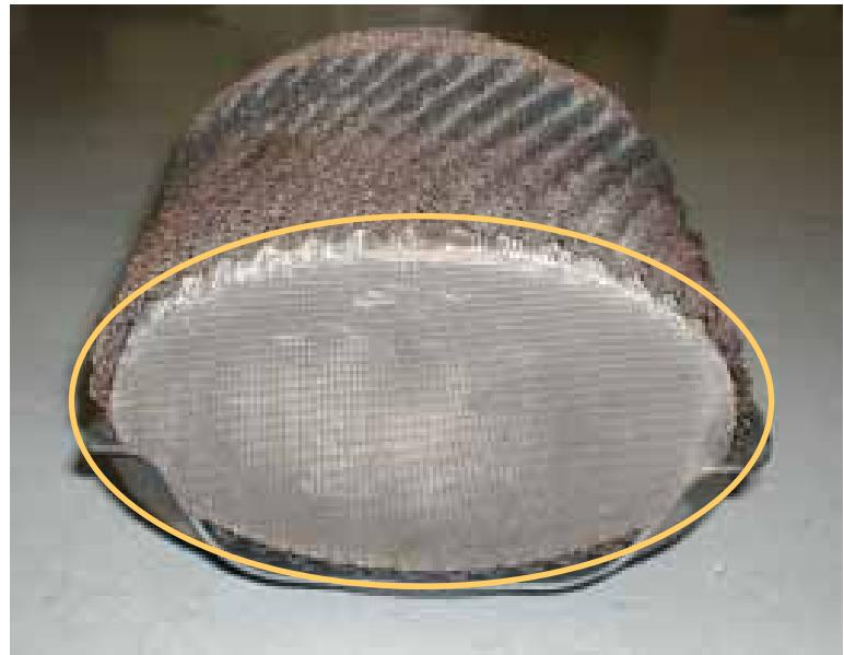
Fig. The innards of catalytic converter
