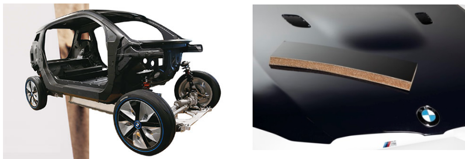
Photo 1-1 CFRP chassis and body panel of BMW i3 [13].
