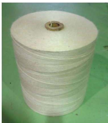
Photo 2-3 Spun jute yarn (Tesac Corp.; K16.5, breached)
