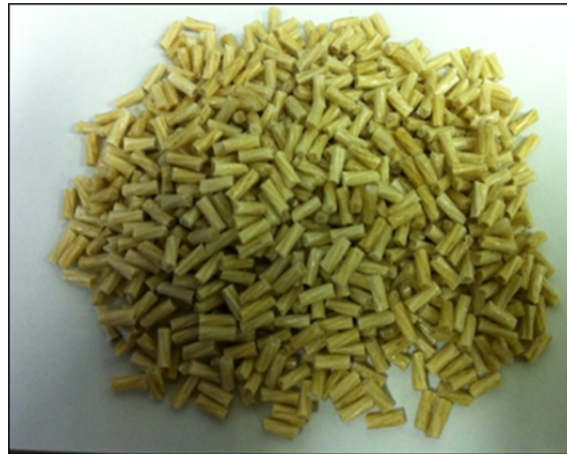
Photo 3-3 The appearance of 50wt%-Jute/PA11 LFT pellets.
