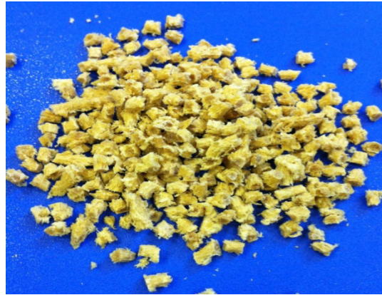
Photo 6-2 The appearance of Jute/PLA fiber-opened pellets, prepared by re-compounding LFT pellets.
