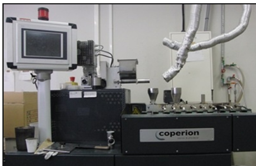
Photo 4-2 Twin screw extruder (Coperion; ZSK18).
