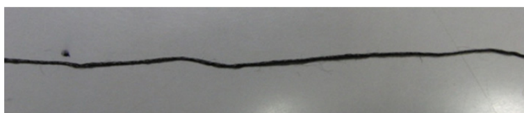
Photo 3-5 Jute fiber yarn heat-decomposed at 220°C for 24hr.
