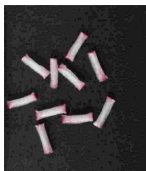
(a) LFT Pellets by KOBE STEEL Process (GF content; 45wt%)
