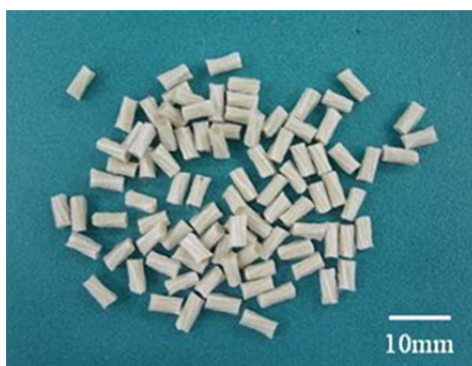
Photo 2-4 The appearance of 50wt%-Jute/PLA LFT pellets.
