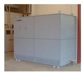
Uses oxidation catalyst and NOx absorber to reduce CVS dilution air concentrations.
