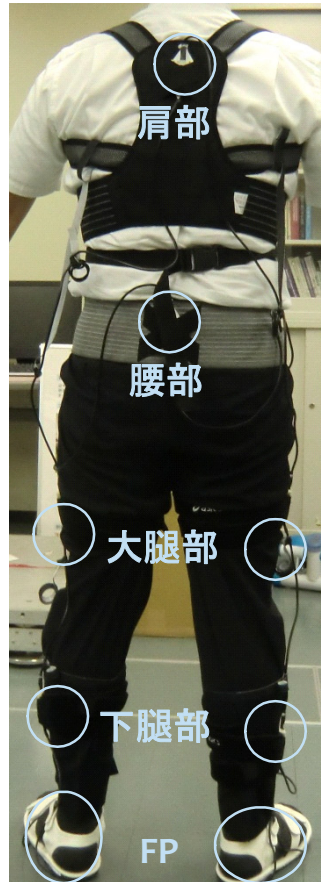
Fig. 3-4 Attached M3D System to Subject
