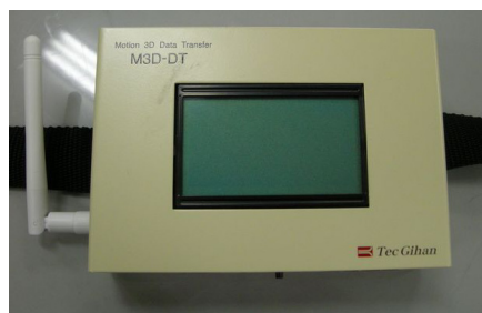
(c) Data Transmitter (M3D-DT)
