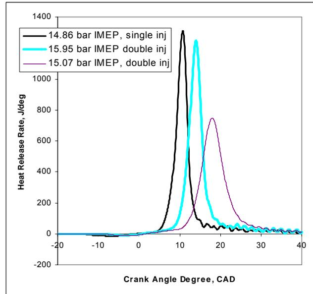
Double injection allows MHRR to be reduced and delayed without increasing cyclic variation and at lower emissions.
