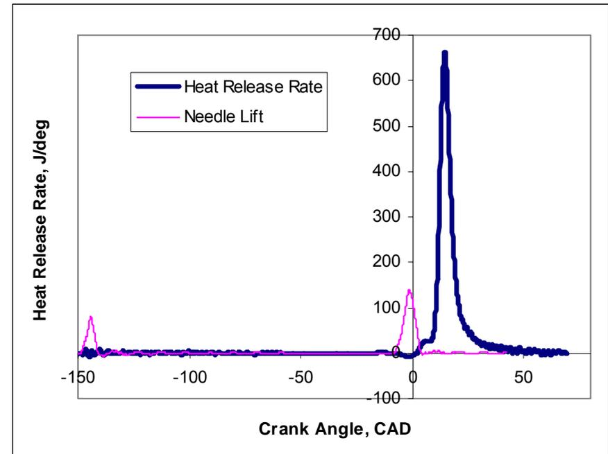
**Gasoline.** Main injection SOI at – 9 CAD. Mean IMEP 12.86 (std 0.108 bar) bar. AVL smoke opacity 0.9%. In g/kWh, ISFC= 174, ISNO<sub>x</sub> = 0.39, ISHC = 6.8, ISCO = 9
