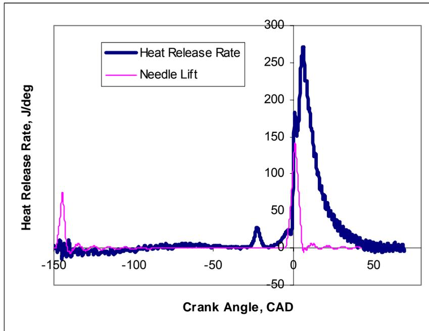
**Swedish MK1 diesel.** Main injection SOI at – 6 CAD. Mean IMEP 11.84 (std 0.115 bar) bar. AVL smoke opacity 8.7%. In g/kWh, ISFC= 183, ISNO<sub>x</sub> = 0.3, ISHC = 11.3, ISCO = 10
