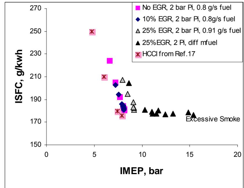
NO<sub>x</sub> increases with IMEP (fuel rate) but can be controlled with EGR. ISFC decreases with IMEP
