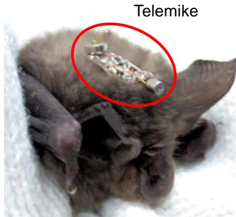
**Figure 3-3** A custom-made telemetry microphone (Telemike) mounted on the *R. ferrumequinum nippon*. The microphone pointed forward and was positioned approximately 1 cm above the noseleaf on *R. ferrumequinum nippon*.
