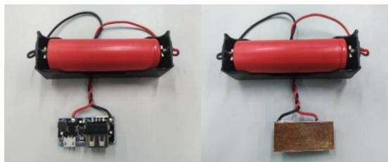
**Fig. 4.17.** Single cell connected with a Custom BMS
