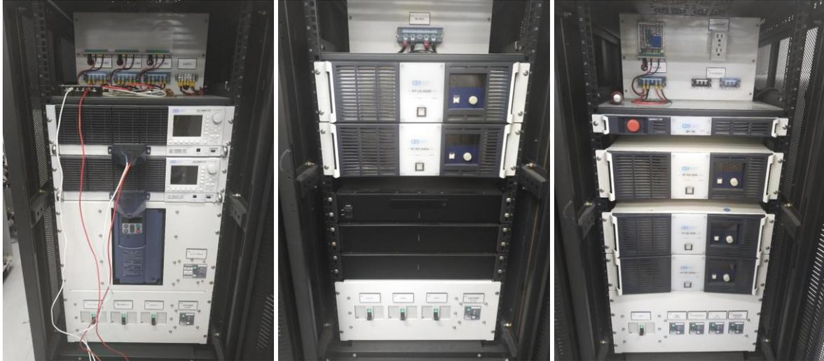
**Fig. A.13.** Devices used for the EV simulation, electronic loads, UPS, DC-DC converters
