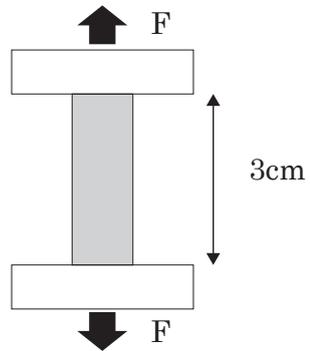
**Figure 1. A schema of the tensile test.**
