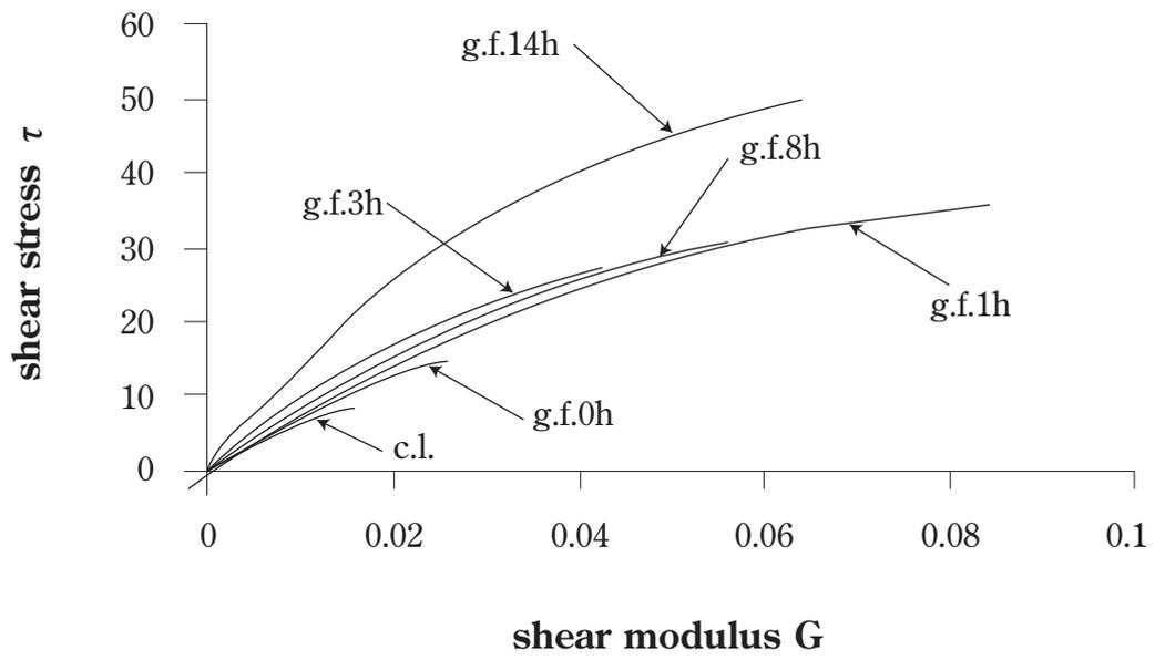
**Figure 10. Representative stress-strain diagrams in the shear test.**
