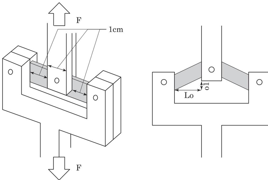
**Figure 2. A Schema of the shear test (A) and a front view (B).**
