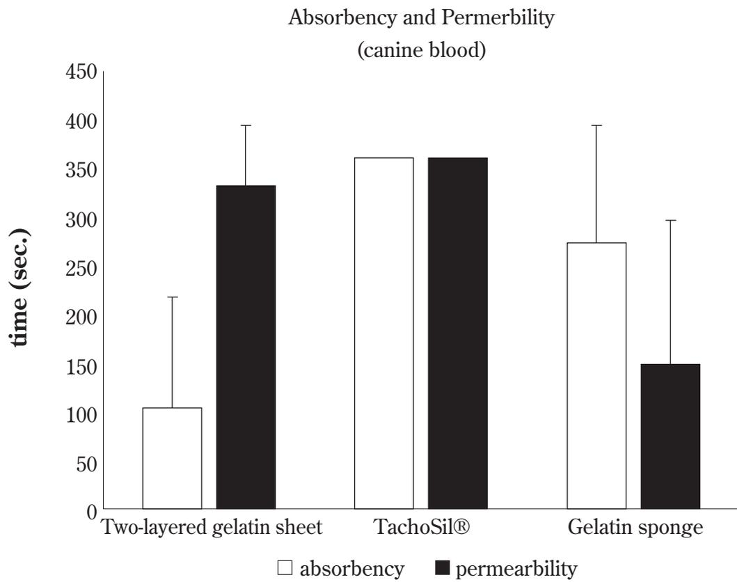
**Figure 3. Absorbency and permeability of the materials**
