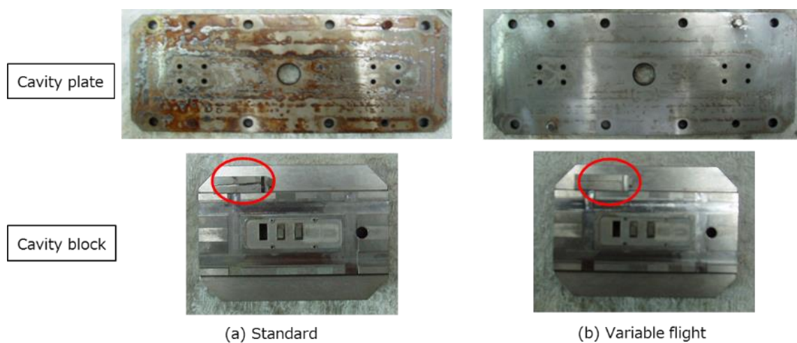
Photo. 3-3 Comparisons of mold stains after injection molding.
