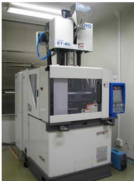
Photo. 4-3 Injection molding machine. (ET-40V TOYO machinery & metal Co., Ltd.)
