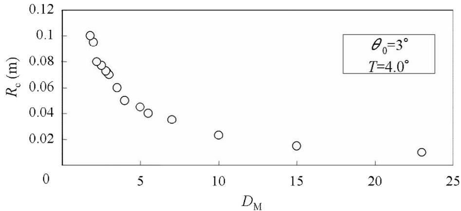
Fig. 2.11 Change of radius by damping
