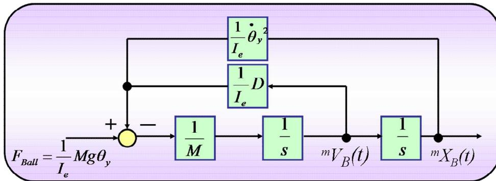
Fig.4.2 Block diagram of motion control of ball
