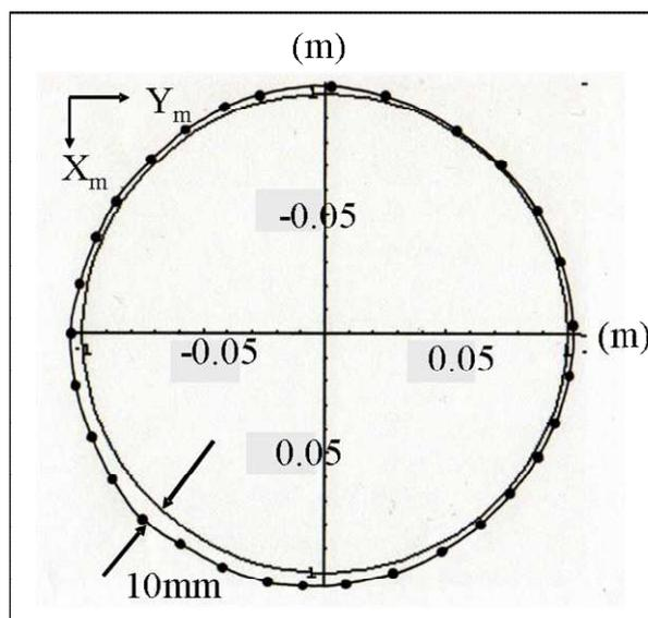
Fig. 2.12 Motion error of rotating ball on a working plate
