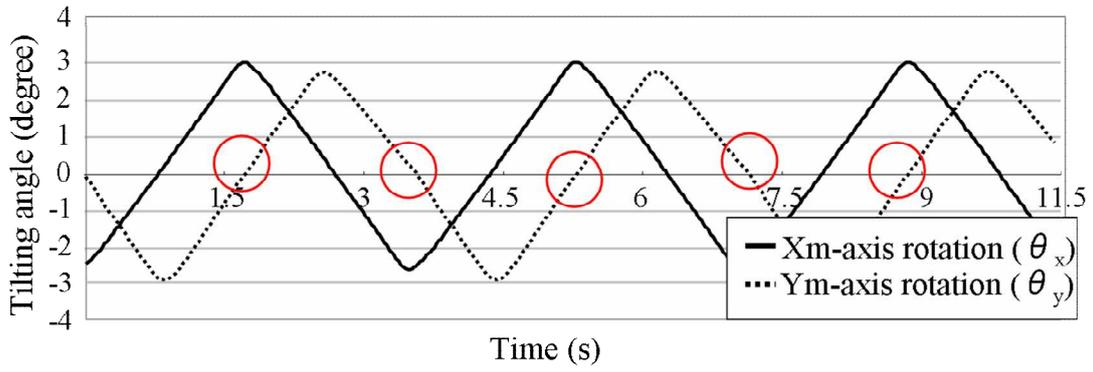
Fig.6.8 Measured tilting angle of working plate by experiment ( $\theta_0=3^\circ$ ,  $T=3.3s$ )
