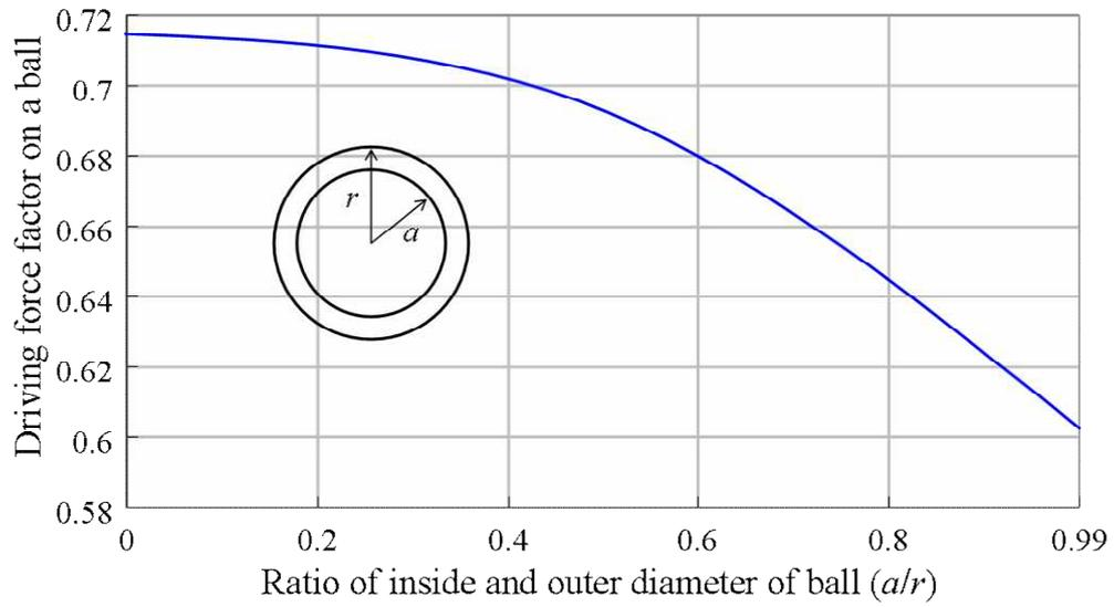
Fig.4.5 Relationship between driving force on a ball and ratio of inside / outer diameter of ball
