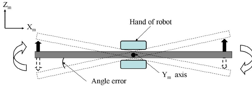
Fig.6.13 Stiffness of supporting plate in  $Y_m$  axis rotation
