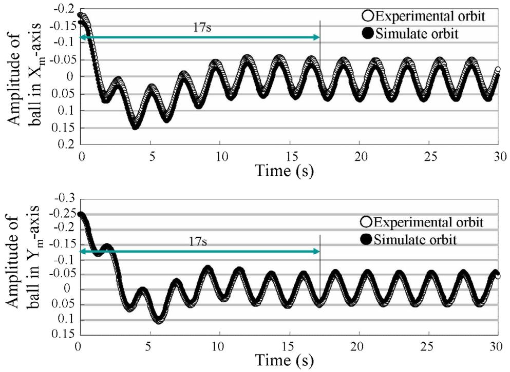
Fig.3.6 Amplitude of ball in  $X_m$ - $Y_m$  axis
