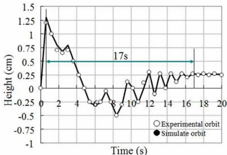
Fig.3.5 Height change of ball at  $Z_m$  direction
