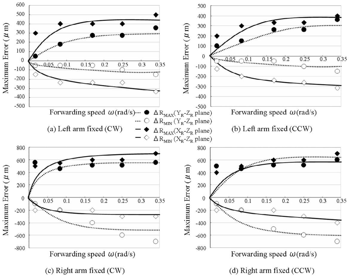
Fig.6.18 Influence of operating speed on DBB maximum error
