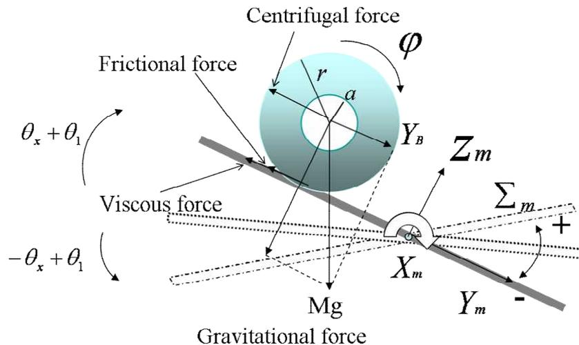
Fig.4.11 Model of ball rolling on working plate with offset angle error
