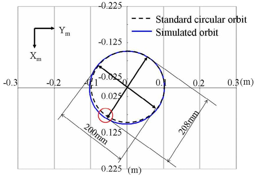
Fig.6.11 Rolling ball path on working plate by simulation
