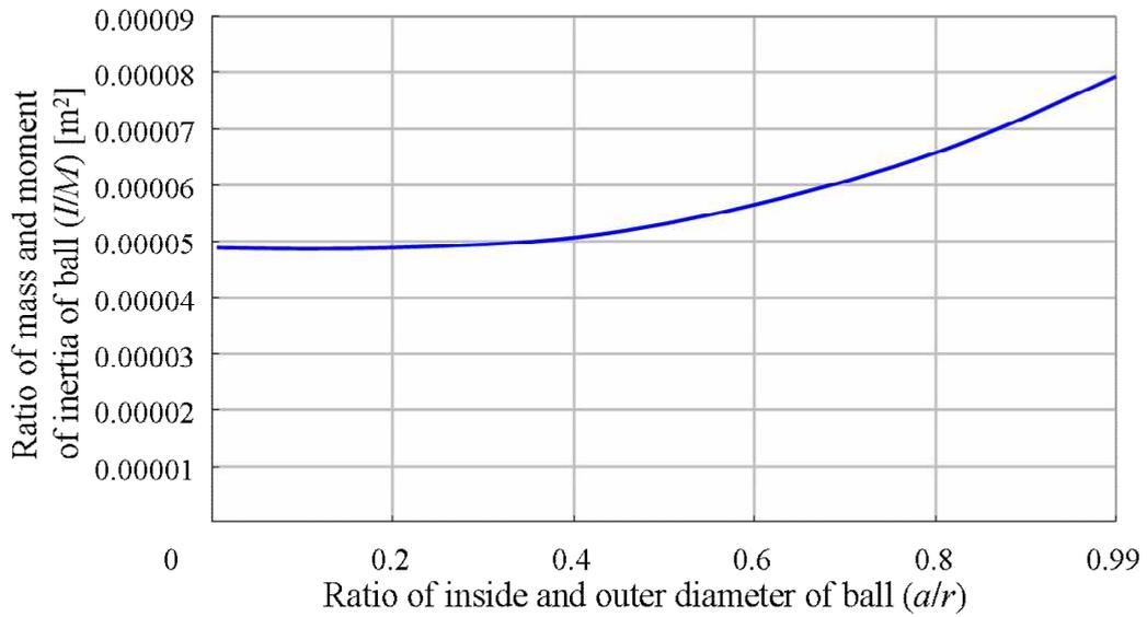
Fig.4.6 Relationship between ratio of  $I/M$  and ratio of inside / outer diameter of ball
