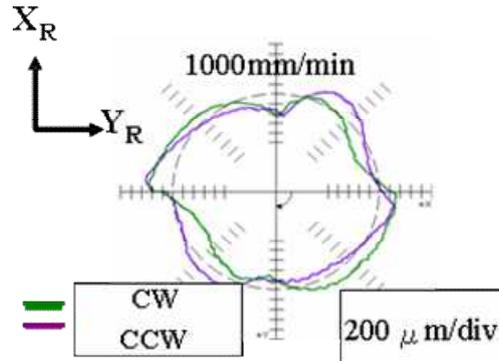
Fig. 2.5 Motion accuracy of robot (dual-arm)
