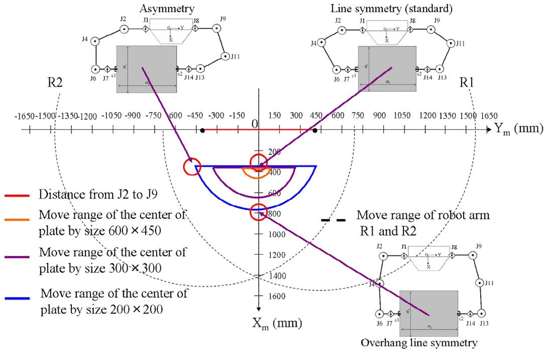
Fig.6.4 Different size plate move range by robot
