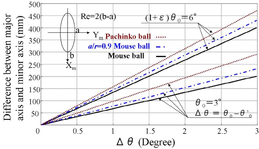
Fig. 4.17 Influence of angle controlling error on circular orbit
