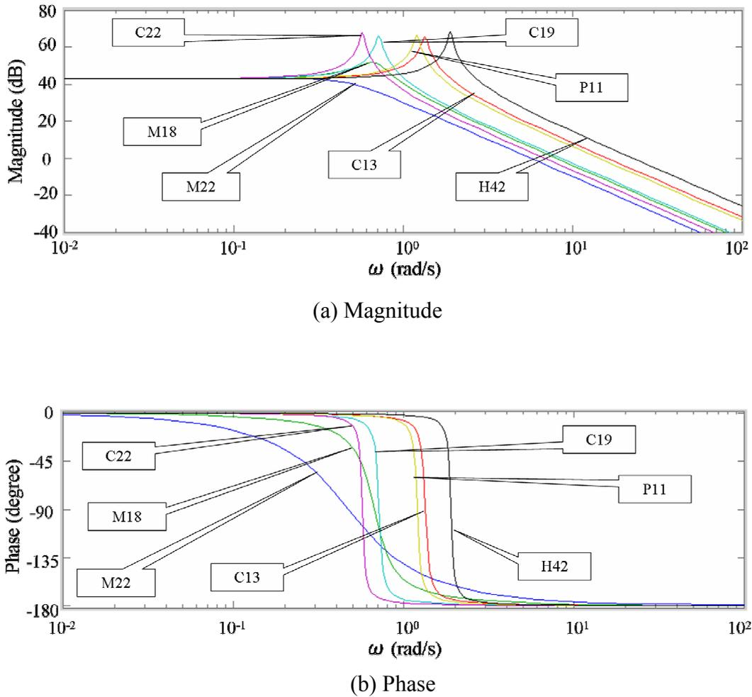
Fig.5.3 Bode diagram of ball rolling motion on working plate
