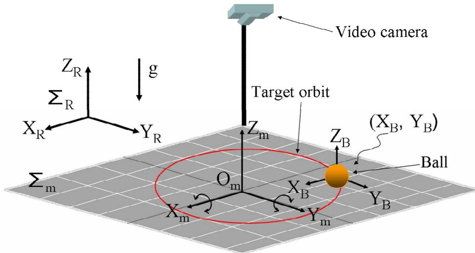
Fig.5.7 Three-dimension model of observing ball rolling on the working plate with video camera
