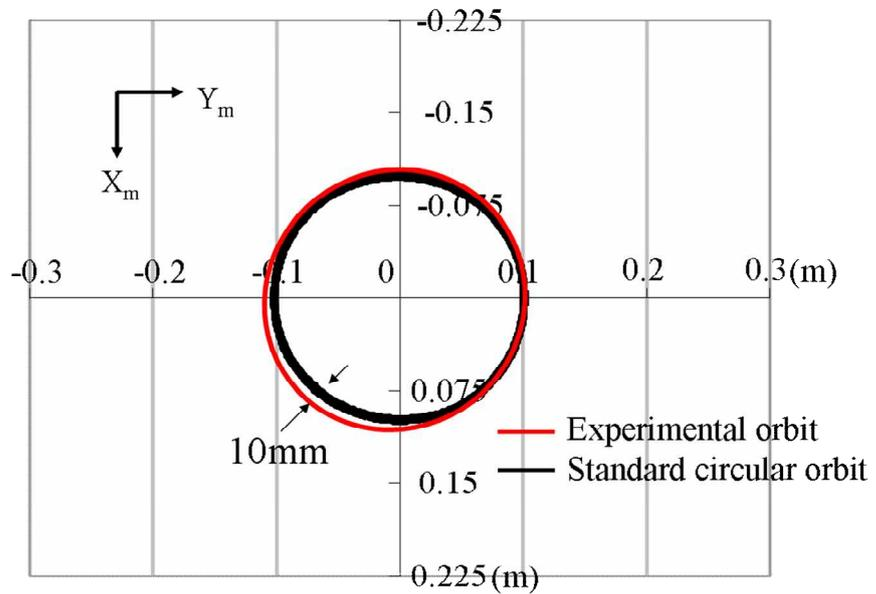
Fig.6.12 Rolling ball path on working plate by experiment
