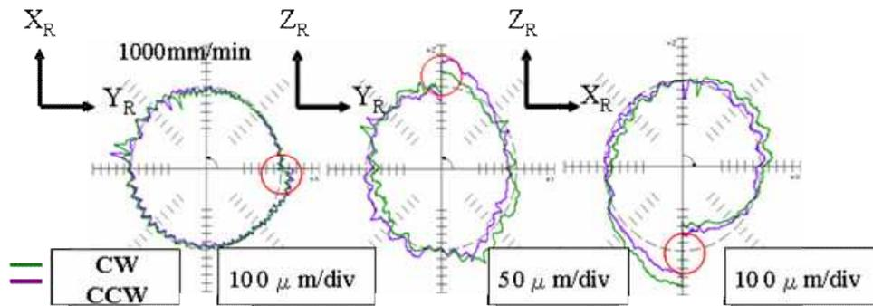
Fig. 2.3 Motion accuracy of robot (left arm fixed)
