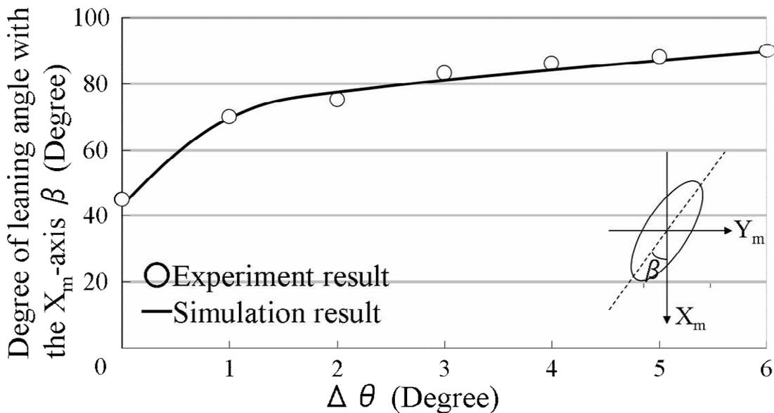
Fig. 3.17 Influence of degree of leaning angle with  $X_m$ -axis on angle and synchronous error
