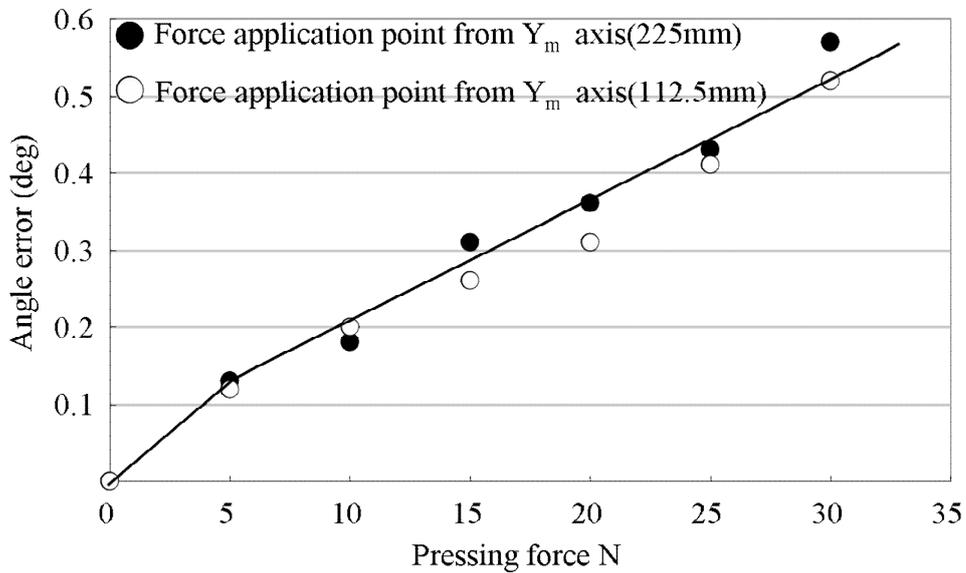
Fig.6.14 Influence of pressing force on angle of plate
