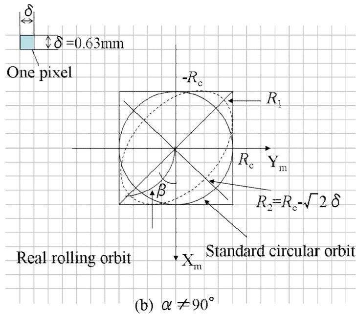
Fig.5.8 Pixel size and error of ball rolling motion on the working plate in image processing
