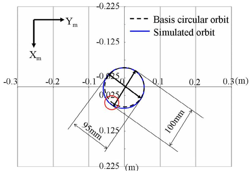
Fig.5.4 Rolling path of simulation result
