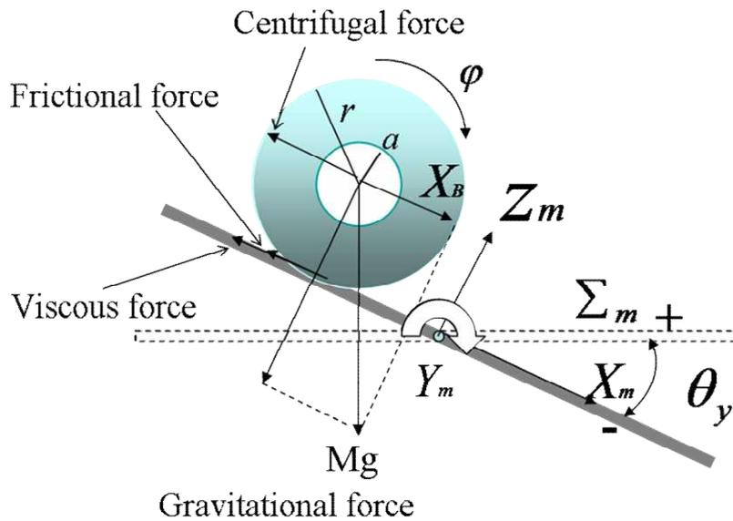
Fig.4.1 Sectional view in two dimensional coordinate plate
