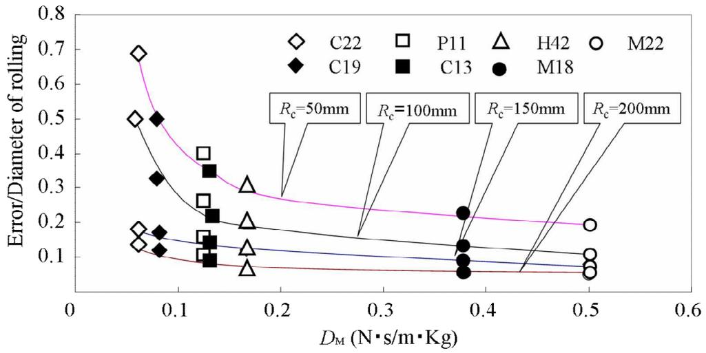
Fig.5.5 Influence of diameter of rolling orbit on maximum rolling error ( $\theta_0=3^\circ$ ,  $T=1.5\sim 4.8s$ )
