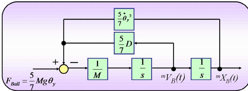
Fig.3.2 Block diagram of motion control of ball
