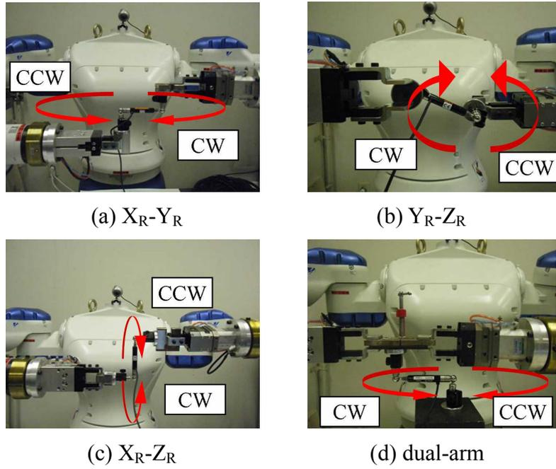
Fig. 2.2 Set up for DBB evaluation (right arm fixed)
