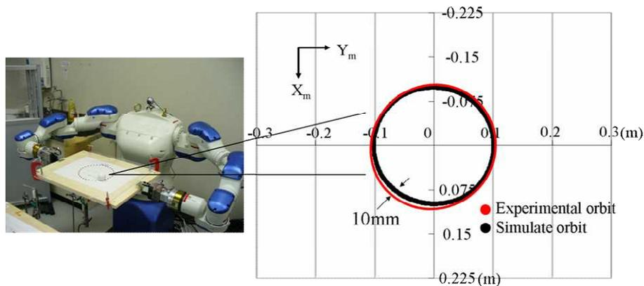
Fig.3.8 Motion error of rotating ball on working plate
