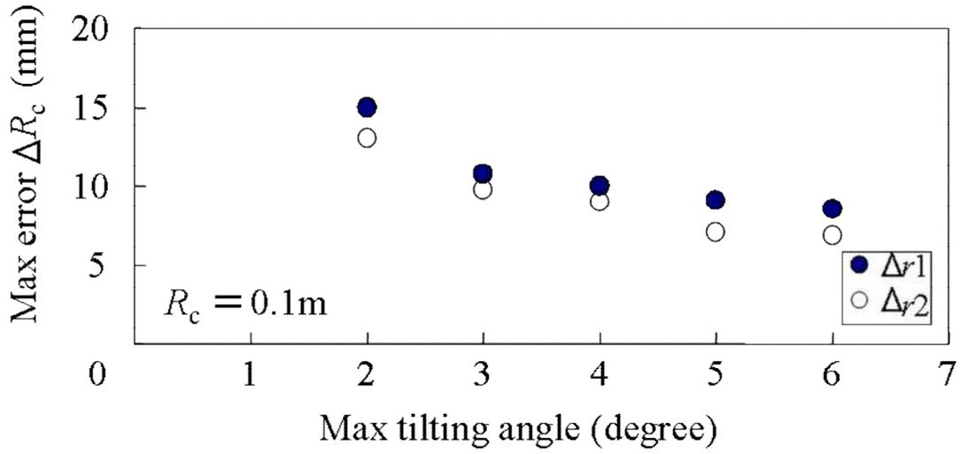
Fig. 2.14 Influence of maximum tilting angle on radius error  $\Delta R_c$
