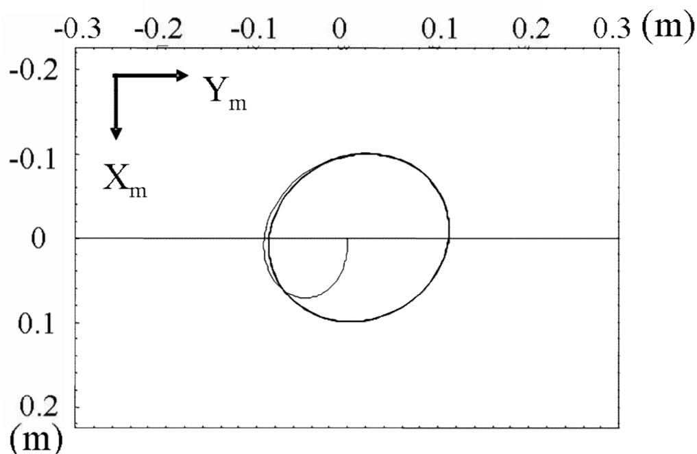
Fig. 2.16 Predicted motion with synchronous error
