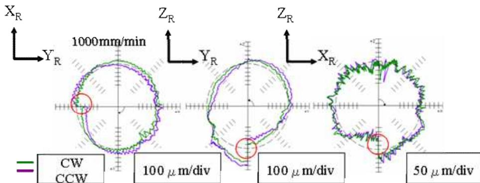
Fig. 2.4 Motion accuracy of robot (right arm fixed)
