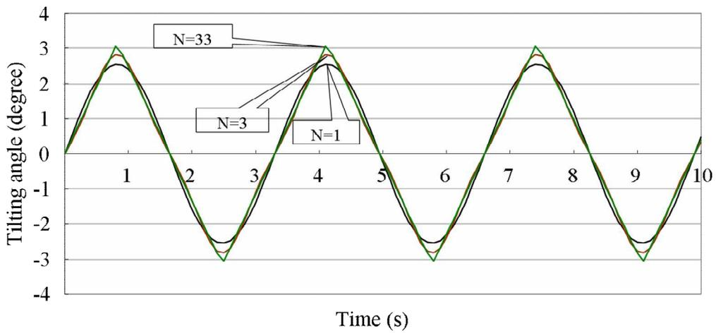
Fig.6.9 Fourier series of triangle wave
