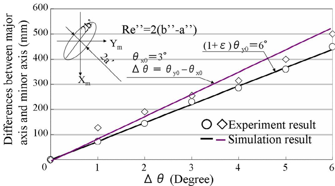
Fig. 3.16 Influence of angle error and synchronous error on circular orbit
