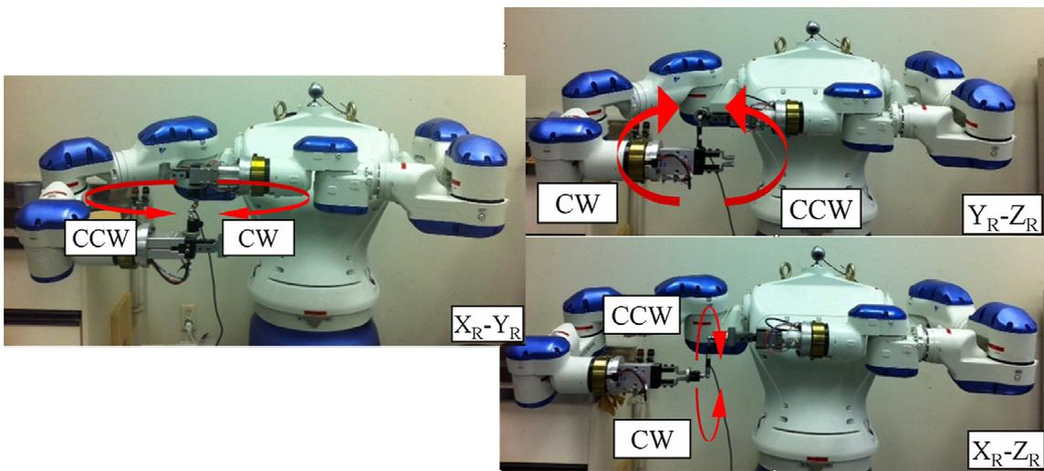
Fig.6.15 Setup for DBB evaluation (left arm and right arm fixed with same pose)
