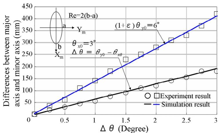
Fig. 3.13 Influence of operating angle on circular orbit
