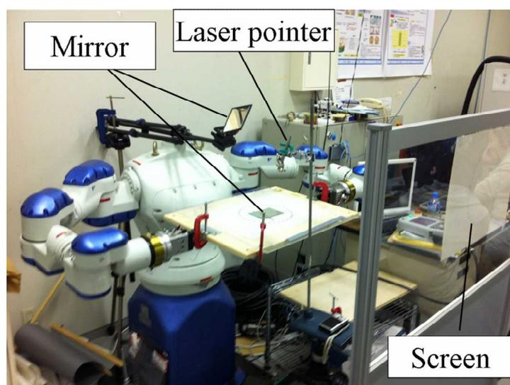
Fig.6.5 Experiment of accuracy measurement of rotational axis with a laser pointer
