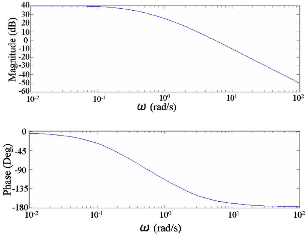
Fig.3.3 Bode diagram of ball vibration on working plate
