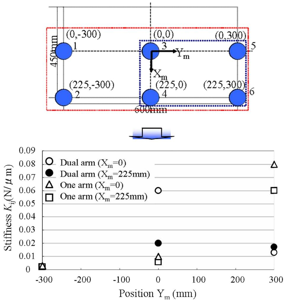
Fig. 2.6 Stiffness of a working plate
