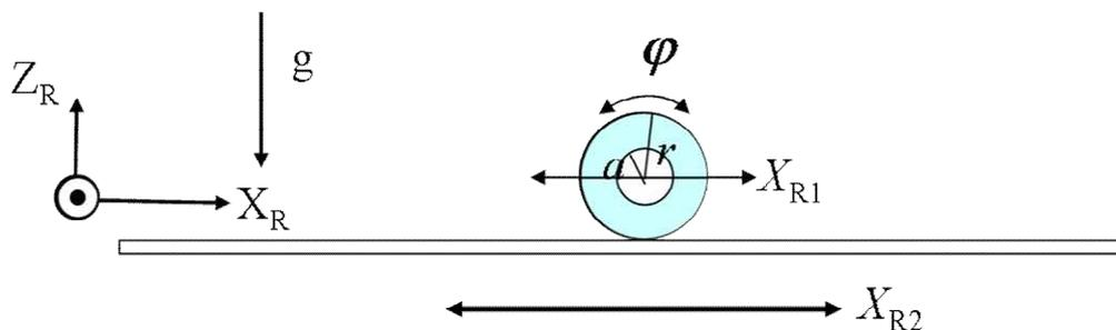
Fig.4.8 Influence of ball by vibration of plate in linear motion on the motion of ball center
