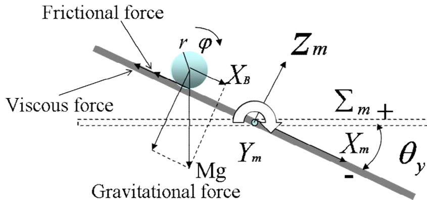
Fig. 2.7 Model of ball rotating on a working plate
