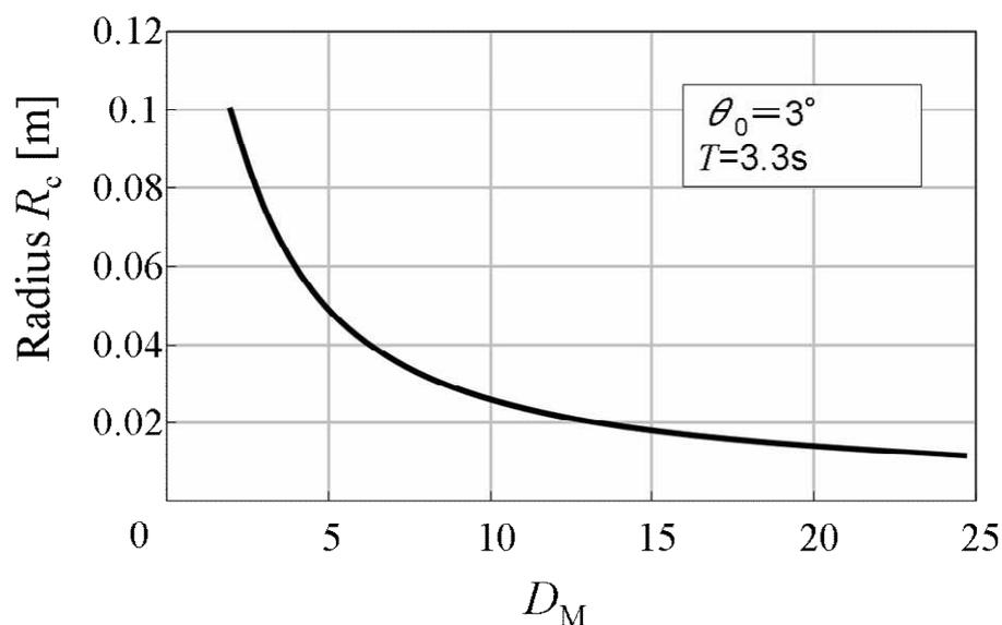
Fig.3.18 Radius change by damping
