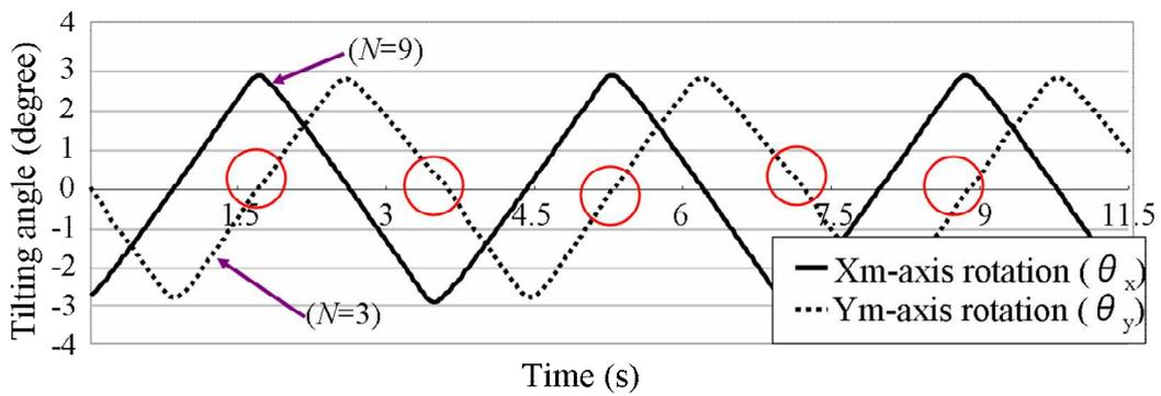
Fig.6.10 Tilting angle of working plate ( $\theta_0=3^\circ$ ,  $T=3.3s$ )
