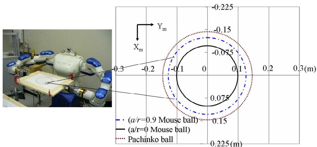
Fig.4.3 Rolling ball path on working plate by simulation
