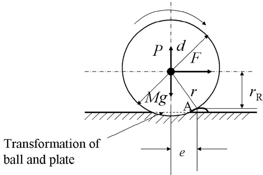
Fig.5.6 Rolling friction model of ball
