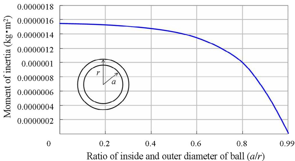
Fig.4.4 Relationship between moment of inertia and ratio of inside / outer diameter of ball
