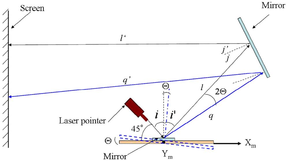
Fig.6.6 Model of accuracy measurement of rotational axis with a laser pointer
