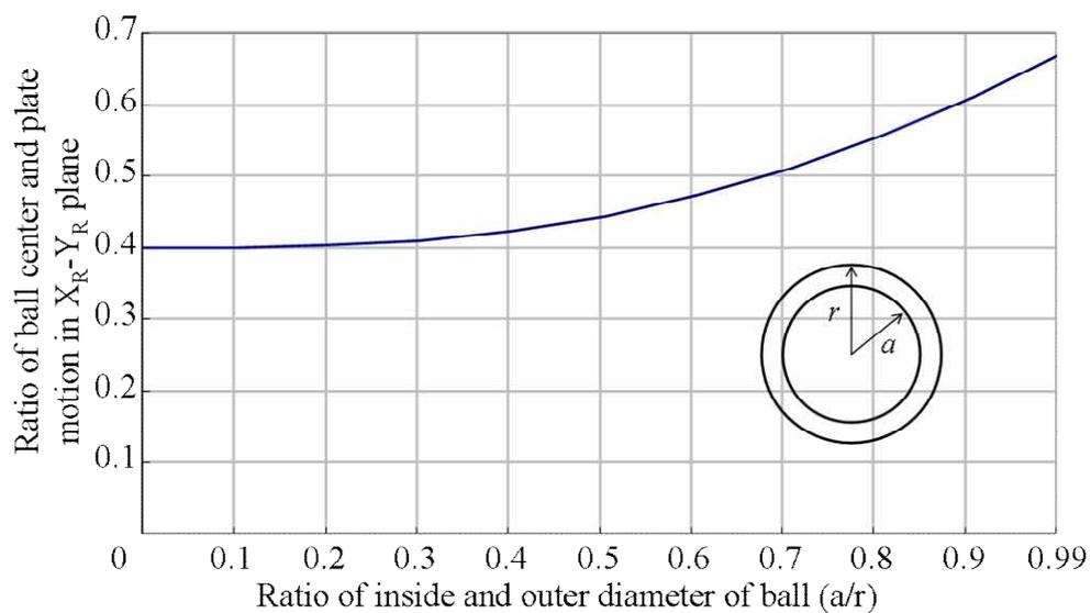
Fig.4.9 Influence of ratio of inside /outer diameter on motion error
